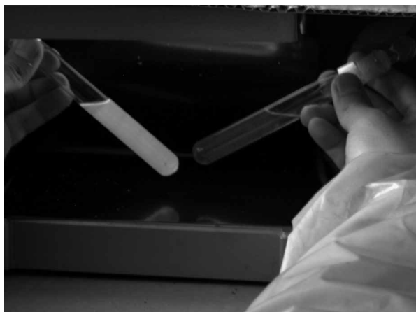
Fig. 5. Left tube: strong fluorescence phenomenon of h-PAMAM in aqueous solution under UV lamp; right tube: pure water.
